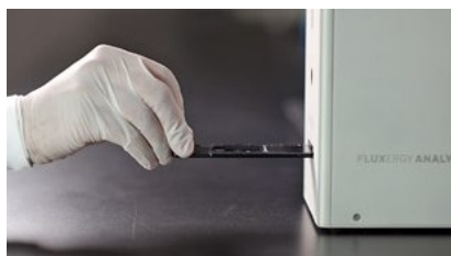
2. Insert Fluxergy Card into Fluxergy Analyzer
