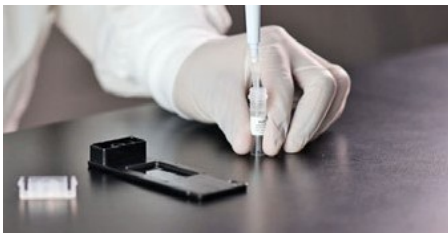
1 . Place Prepared Sample into Fluxergy Card
