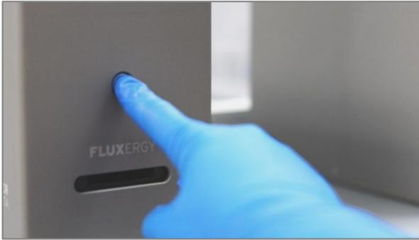
Turn on the Fluxergy Analyzer by connecting the power cord to the AC/DC port found on the back of the analyzer. Press the power button on the device. The Analyzer can remain ON when not in use. The Analyzer must be on to be found by Fluxergy Works.
