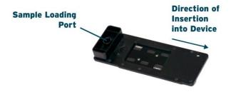
The Fluxergy PCR Card is a disposable card into whichthe PCR reagents mixed with test samples are manually pipetted in. Each card contains a single sample/reagent input well and microfluidicchannels that control the flow of liquid, and reaction wells. The Fluxergy PCR Card is self- contained to prevent cross-contamination between samples.
